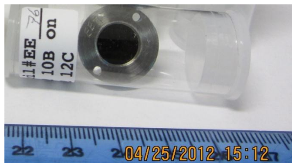
Figure 3: Unsupported 100 µg/sq.cm Boron-10 on 60 µg/sq.cm Carbon-12.
