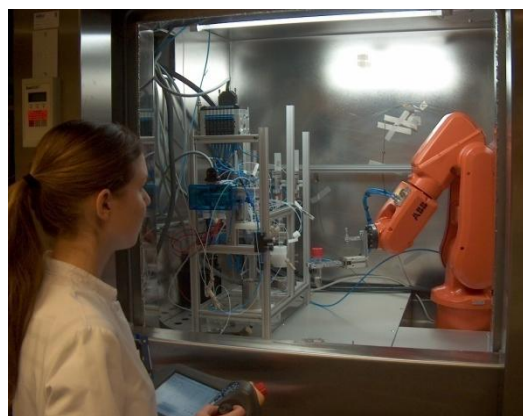
Figure 1: Target handling inside the hot cell using ABB IRB120 robotic arm.
