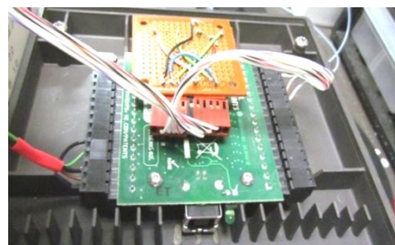
Fig. 1: Photo of DAQ hardware mounted under EM-1's cover. Relay driver circuit is under brown proto-board.
