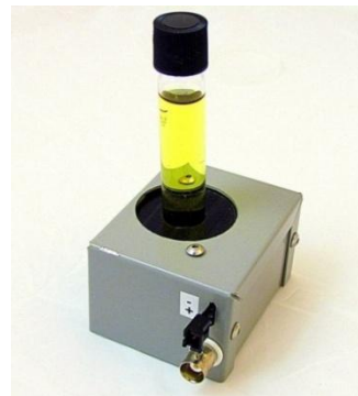
Figure 1: Simple spectrophotometer based on an LED light source and Photodiode.
