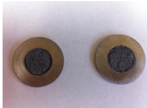
Figure 1: ^{100}\text{Mo} -targets prepared by EPD / sintering
