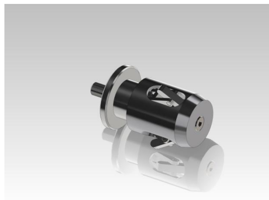
Figure 2: SolidWorks® 3D-drawing of locking mechanism for target pick-up.
