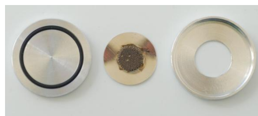
Figure 2: Opened target left: Al disk with O-ring, ^{64}\text{Ni} on Pt foil, right: Al lid with 10 mm hole.
